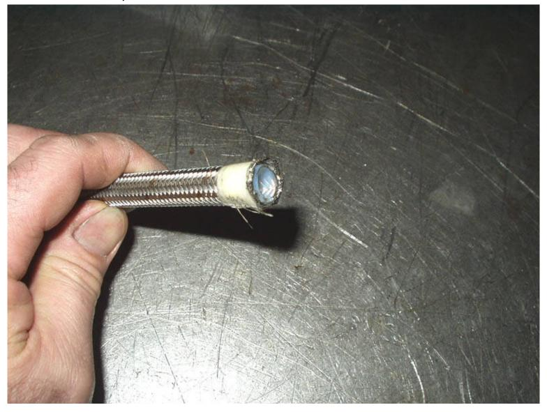
**Step Three**: Slide the female hose-nut down onto the hose with the threaded opening oriented towards the cut hose end. Carefully remove the tape from the stainless over-braid. Now take a blunt tipped screwdriver or alternate tool and spread the stainless over-braid away from the inner Teflon hose liner about a 1/4".
