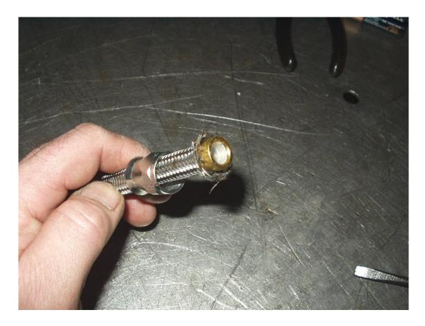
**Step Six**: Grab a suitable tapered punch and expand the Teflon liner into the I.D. of the ferrule firmly.
