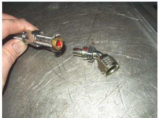
**Step Eight:** Grab the hose end and firmly insert it into the female hose end. You may at this point pull the hose end back out to make sure that the Teflon hose liner has not folded over or been injured in any way during the hose end insertion process, then pop it back in after all is verified as proper.
