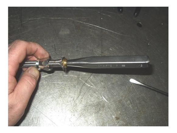
**Step Seven**: Put a few drops of your favorite lube on the hose end male nipple, the threaded area of the hose end, and a drop also in the female hose end to aid assembly and prevent thread galling while tightening. (Any lube will essentially do, though we prefer to use moly based lube, cam / lifter assembly lube works great).
