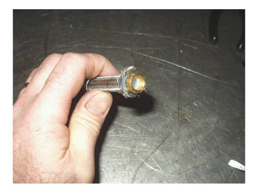
**Step Five:** Grab the hose and push it firmly against a solid surface to push the Teflon liner all the way into the ferrule until it seats against the flat inner stop.
