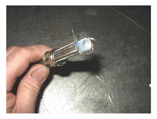
**Step Four**: Carefully start the brass ferrule onto the Teflon liner. The Teflon liner is to go inside of this ferrule. Be careful not to let the Teflon liner fold over or distort during this step.
