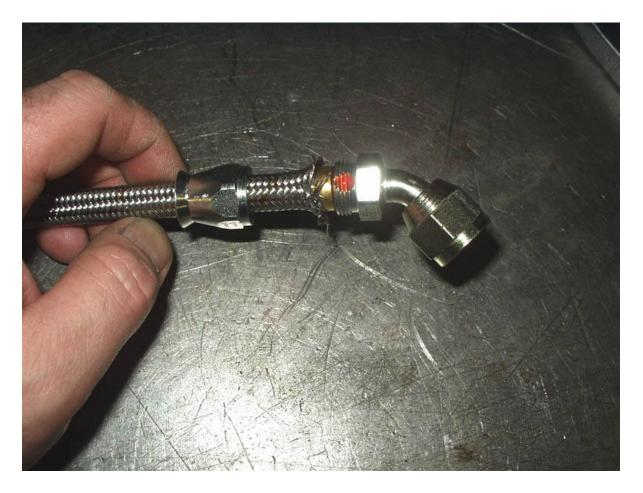
**Step Nine**: Slide the female hose nut firmly up and over the necked out stainless hose over braid until you can get the hose end threaded into the nut - be careful not to cross thread these two items.
