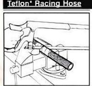
Step 1. Cut hose square to length with fine-tooth hack saw or cut-off wheel. To minimize wire braid flare out, wrap hose with masking tape and cut through tape. Remove tape, trim loose wires and flush with lube before next step. Burrs on bore of tube should be removed with a knife, Clean the hose bore.
